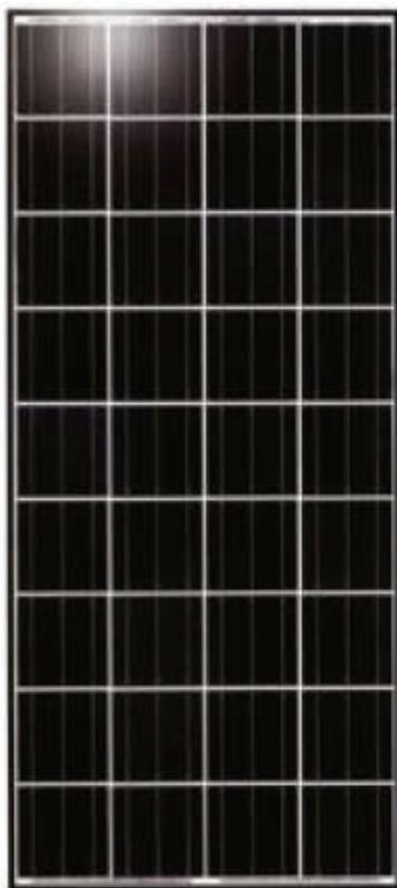
The SPA 260 photo voltaic Solar Panel is an ATEX Ex nAC certified product for Zone 2 gas hazardous area applications. The cells of the panel are encapsulated between a tempered glass cover and EVA pottant to provide maximum protection in the most extreme environmental conditions.
