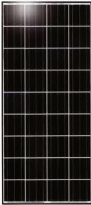
The SPA 130A photo voltaic Solar Panel is a Zone 1 ATEX Ex mb e certified product. The cells of the panel are encapsulated between a tempered glass cover and EVA pottant with an aluminium polyester protected back sheet to provide maximum protection in the most extreme environmental conditions.
